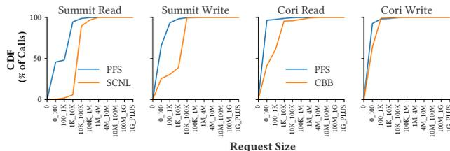
**Figure 4: Cumulative distribution functions (CDF) for the number of requests in a given Darshan bin size for reads (left) and writes (right) in Summit and Cori's in-system layer and the parallel file system.**
