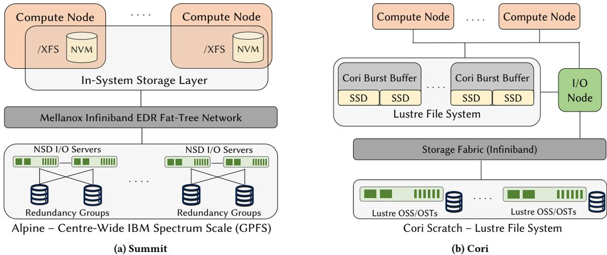
**Figure 1: I/O subsystem architecture for Summit and Cori. Both systems consist of two storage layers: an in-system layer and a parallel file system (PFS) layer, where the in-system layers are compute-node local (Summit) and system-local (Cori) and the PFS layers are IBM Spectrum Scale – GPFS (Summit) and Lustre (Cori) deployments (§2.1).**
