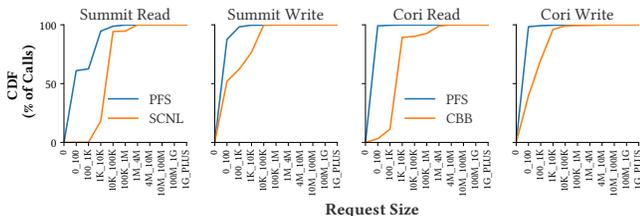
**Figure 5: Cumulative distribution functions (CDFs) for read (left) and write (right) requests on Summit and Cori's in-system layer and the parallel file system. The analysis is similar to Figure 4 but only for large jobs (i.e., number of processes > 1,024).**
