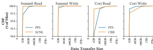
**Figure 3: Cumulative distribution functions (CDF) for the number of files in a transfer-size bin for read (left) and write (right) in Summit and Cori's in-system layer and PFS. We define data transfer size in §3.1.**
