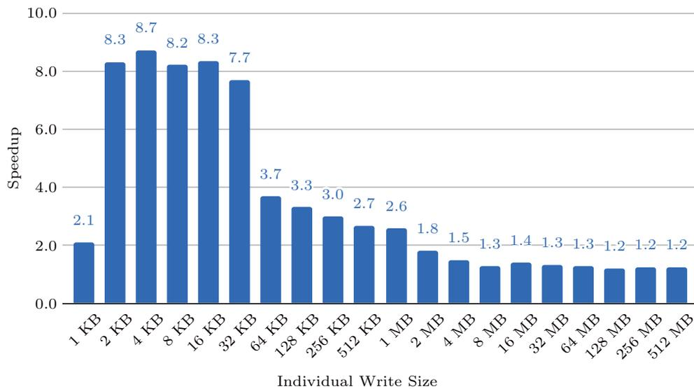
Fig.14. Speedup of SWMR over non-SWMR in writing dataset with different write sizes.
