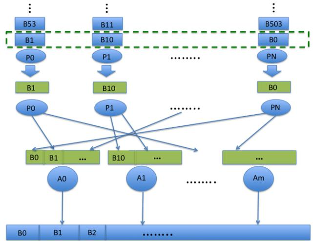
Fig. 3. Illustration of collective buffering. Chombo first copies the data on a box (denoted by  $B_0, B_1, \dots$ ) into a 1D buffer (green), and then sends these buffers to HDF5. In collective buffering, aggregators ( $A_0, A_1, \dots$ ) collect the data sent by each of the processes ( $P_0, P_1, \dots$ ) into buffers (in green) to write out as many contiguous chunks as possible. Note that aggregators only have access to a subset of all the boxes at a time in this implementation of Chombo.
