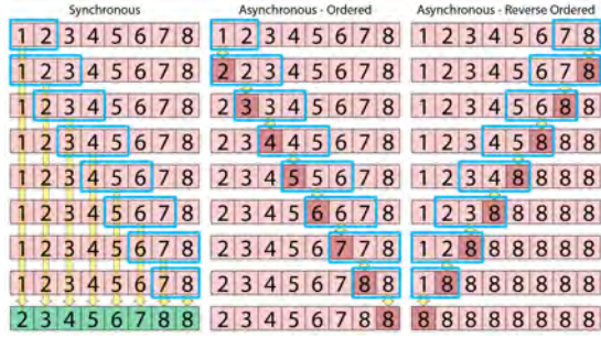
Figure 2: Comparison of synchronous and asynchronous updates of a 1D cellular automaton. The illustration shows only the first iteration in detailed steps. In the synchronous case, the original buffer is in red and the extra buffer for intermediate results is in green. Values are updated according to the maxima within the moving window (in blue), indicated by the yellow arrows. In the asynchronous cases, there is no extra buffer, so updates are immediate. The updated values in each step when the window moves are in dark red. We can repeat the iteration for the first two cases until all cells are updated to the maximum ID. Their results look exactly the same. The last case has already converged after the first iteration.
