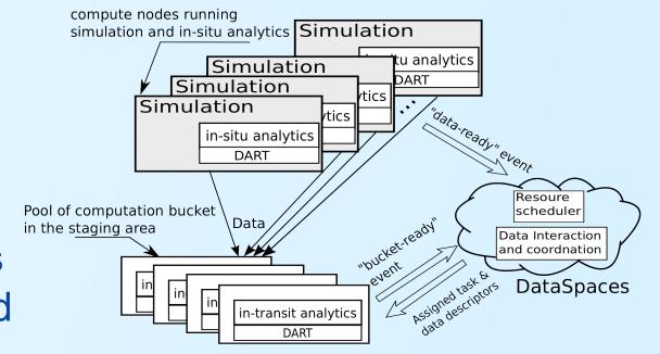
abstraction derives from the tuple-space model and can be associatively accessed by the interacting applications of a simulation workflow (right).
