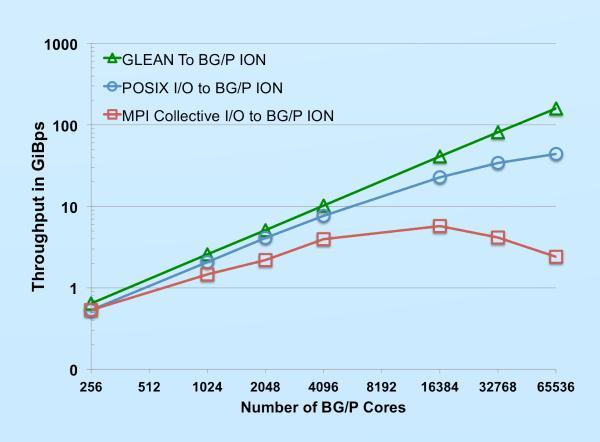
Strong scaling performance for 1GiB data movement off ALCF Intrepid Blue Gene/P compute nodes. GLEAN provides 30-fold improvement over POSIX I/O at scale. Strong scaling is critical as we move towards systems with increased core counts.
