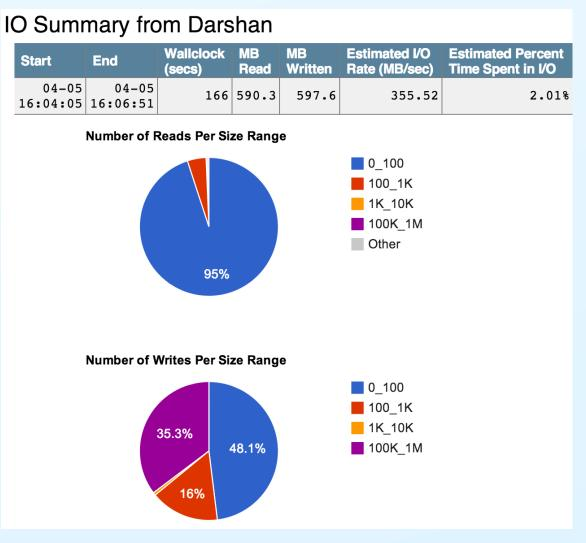
Example of NERSC web portal data available to Hopper endusers once a job has completed. Darshan data is used to automatically produce a graphical summary indicating the access size distribution, the amount of data accessed, estimated performance, and percentage of time spent performing I/O. Users can use this data as a starting point to evaluate I/O performance and validate application behavior.
