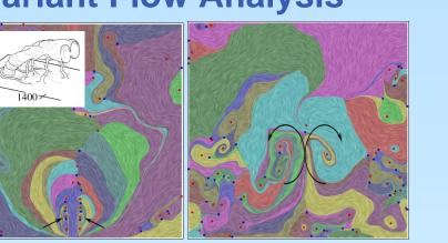
flow shows the presence of jet-shear vortices
