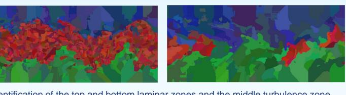
Identification of the top and bottom laminar zones and the middle turbulence zone is heavily influenced by perturbation. Numerical noise (left) is removed (right), a small perturbation having drastic effects on the segmentation.
