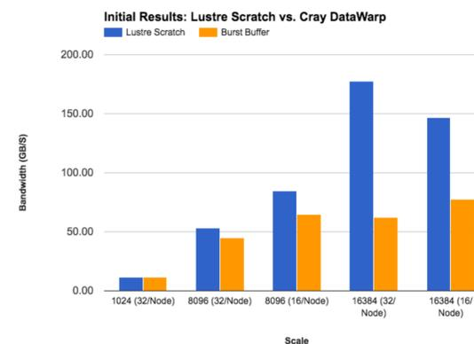
Fig 3. Comparison of I/O initial performance for the VPIC-I/O kernel on the Cori PFS and Cori Burst Buffer.
