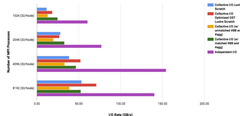
Fig 5. Performance comparison with several I/O configurations on both the Cori PFS and Cori Burst Buffer System. Blue & Red: MPI-IO collective runs on PFS. Yellow & Green: Matched & Unmatched Numbers of MPI-IO Aggregators to Burst Buffer Nodes. Purple: Independent I/O
