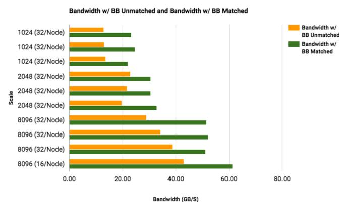
Fig 4. I/O performance (I/O rate in GB/s) on the Cori Burst Buffer with matched and unmatched numbers of BB nodes and MPI-IO aggregators
