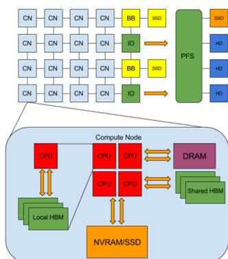
Fig. 1 The figure above is an abstract diagram of a HPC equipped with non-volatile storage in its various forms. The phase 1 Cori Supercomputer is equipped with BB nodes (in yellow) but not node local NVRAM.
