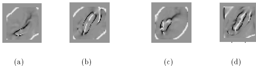
Figure 4: Maximum principal curvatures of surface intensity for pistachios: (a) & (b) clean and (c) & (d) infested
