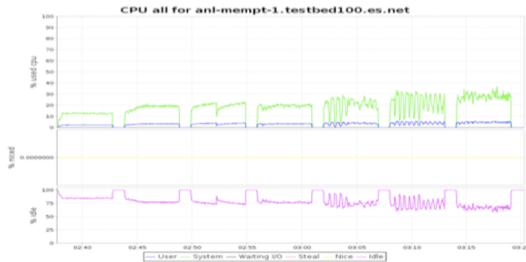
Figure 8: ANI testbed 100Gbps (10x10NICs, three hosts): CPU utilization vs the number of concurrent transfers [1, 2, 4, 8, 16, 32, 64 concurrent jobs - 5min intervals], TCP buffer size is 50M
