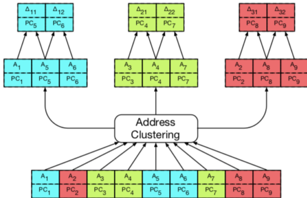
(a) Clustering the address space into separate streams.
