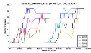
Fig. 5. Number of streams used for slow client side adaptation
