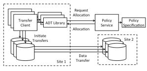
Fig. 1. Service interactions for bulk remote data access use cases.
