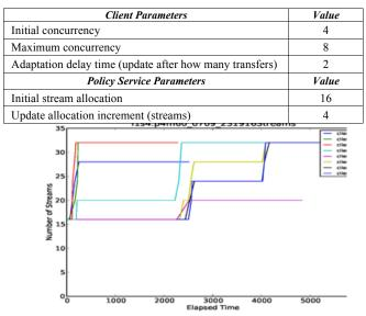
Fig. 8. Stream allocation for fast increases in policy service allocation
