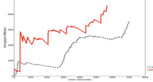
Fig. 9. Comparison of adaptive vs. non-adaptive data transfer performance for a 260 GByte data set from NISN to NERSC.
