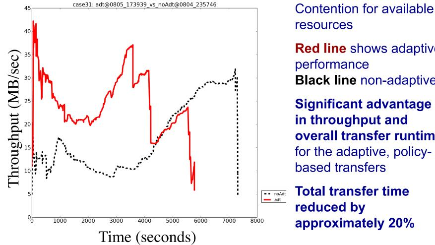
**Red line** shows adaptive performance Black line non-adaptive Significant advantage in throughput and overall transfer runtime for the adaptive, policy-
